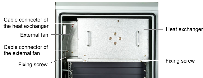
Figure 5-7 Positions of heat exchanger and external fan
